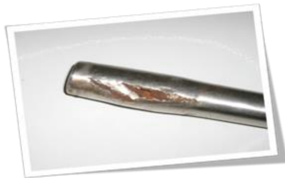
Figure 1. Mechanical and magnetic failure of a low-cost finger magnet
